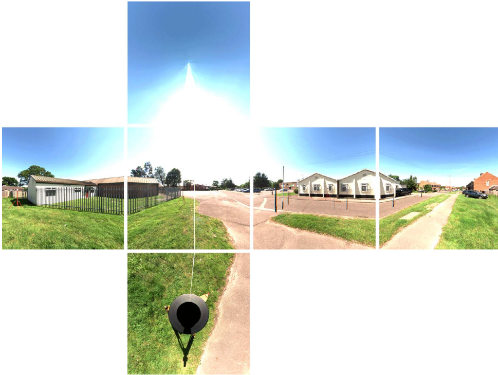
Figure 2. Tone mapped example of the cubic projection of an HDR image from the SYNS dataset.
