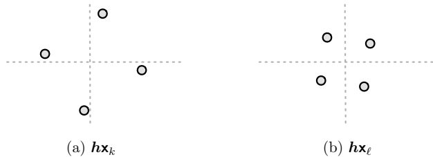
Fig. 1: Complex plane representation of the four values of \mathbf{h}\mathbf{x} for a given \mathbf{h} and a given quartet, with the ADC quantization boundaries indicated by dashed lines. Left-hand side, for \mathbf{x}_k , which has a larger magnitude but worse orientation. Right-hand side, for \mathbf{x}_\ell , which has a smaller magnitude but better orientation. On this channel, quartet k yields a higher mutual at low SNR while quartet \ell yields a higher mutual information beyond the low-SNR regime.
