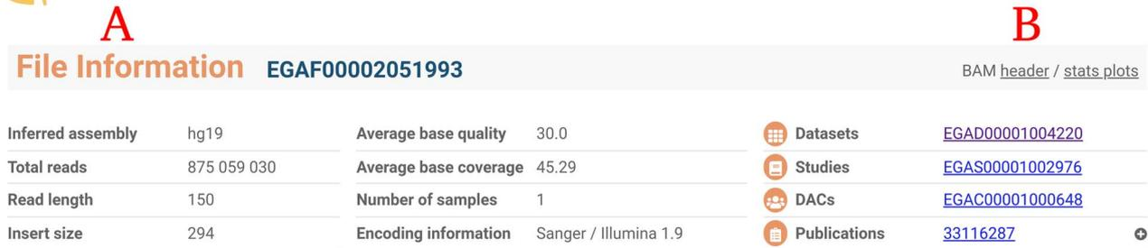
**Figure 2.** QC File Information section for a BAM file from H3AFRICA TRYPANOGEN2. (A) File Information section with general data about the bam file. (B) Link to bam header and plots generated by bamstats plot plugin from SAM tools (<https://filesportal.ega-archive.org/EGAF00002051993>).
