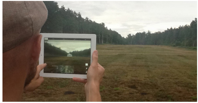
Figure 2: Through the hand-held device, user can see virtual reconstruction placed in real world coordinates.
