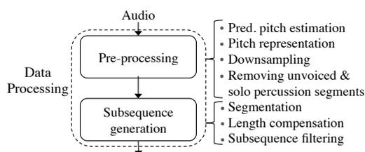
Figure 2. Block diagram of the data processing module.
