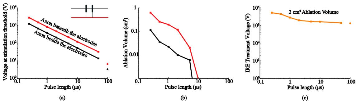
**Figure 5:** (a) Voltage stimulation thresholds versus pulse length for two different locations of the nerve fiber (see figure 2) when bursts of bipolar pulses with a total energized time of 100  $\mu$ s and with a 2  $\mu$ s
