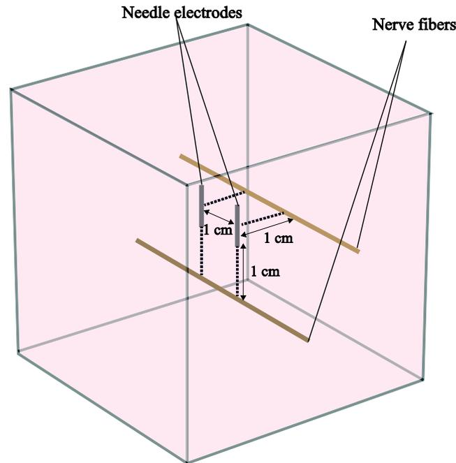
**Figure 3:** Model geometry used in the present study to simulate excitation of long nerve fibers (=myelinated axon). Two nerve fiber locations are analyzed: first, an axon parallel to the axis that joins the centers of the electrodes at a distance of 1 cm from them. Second, an axon inside the plane defined by the electrodes at a distance of 1 cm underneath them.
