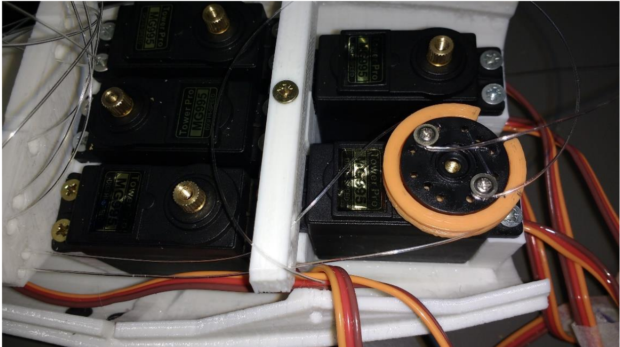
(Figure 11: A Servo-rotor wheel fully tightened and attached to the servo-motor, all attached to the servo-bed.)
