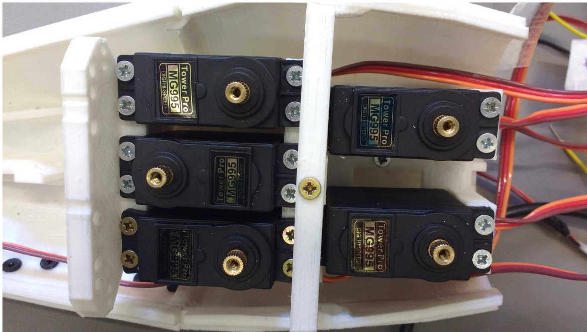
(Figure 5: Servo bed from above, note the cable positioning)
