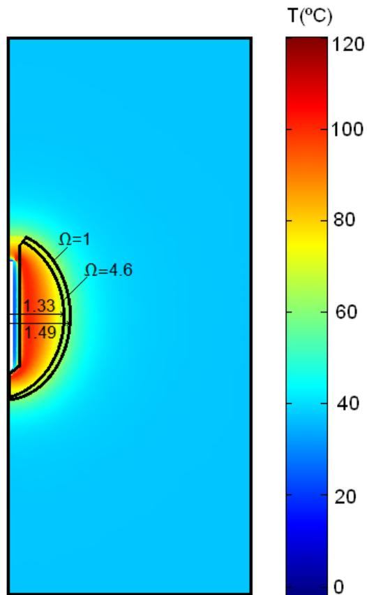
**Figure 5** Temperature distributions after 12 minutes of RF ablation and previous application of electroporation pulses. The black lines represent the thermal damage lesion which corresponds to  $\Omega=1$  and  $\Omega=4.6$ . The values of the minor transverse lesion diameters (in cm) are shown for both contours of thermal damage.
