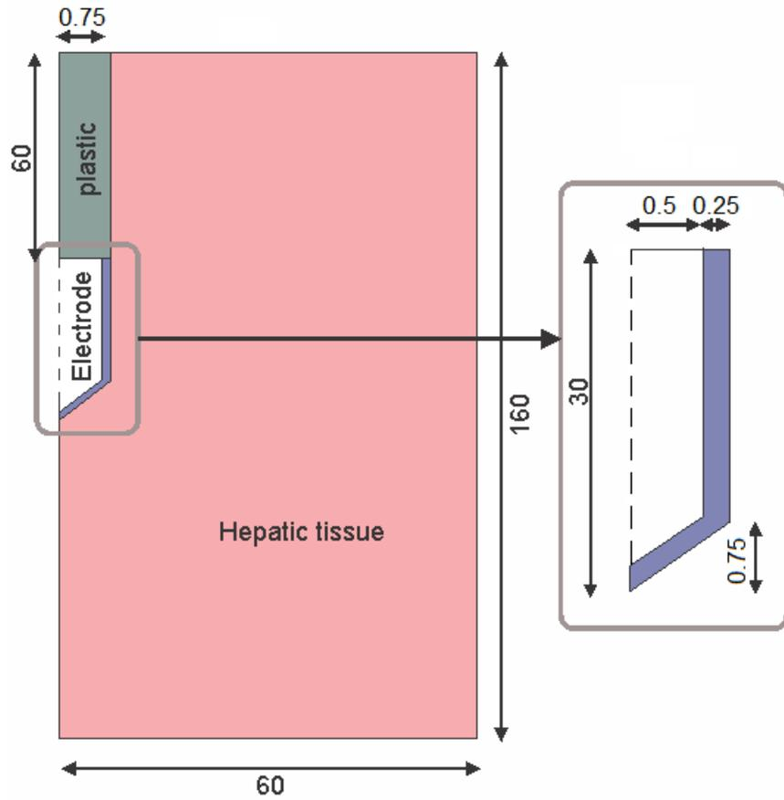
**Figure 1** Geometry of the two-dimensional model used in the theoretical study (out of scale, dimensions in mm). The domain is divided into three zones: plastic portion of the electrode, metallic electrode and hepatic tissue.
