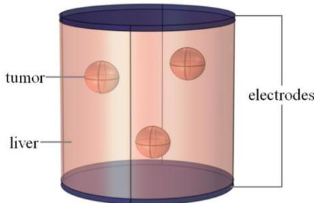
Fig. 2 Geometrical model used in the numerical study. The model included three different elements: metallic electrodes, hepatic tissue, and tumor tissue.
